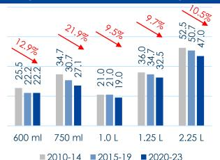
Plastic usage reduction through light weighting of Preforms and Closures for PET bottles.
