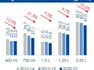
Plastic usage reduction through light weighting of Preforms and Closures for PET bottles. Phasewise implementation of certain SKUs is under process
